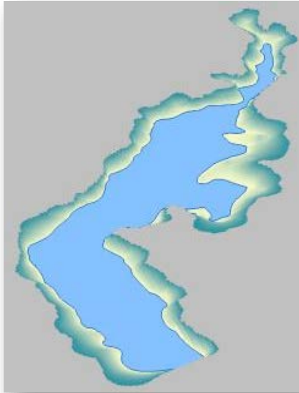
Predicted water surface (blue) under a 5.0-ft drawdown scenario. Although minor ponding would be expected in isolated areas that poorly dewater, most of the aquatic habitat within the pond would remain connected. Figure provided by SDRA.
